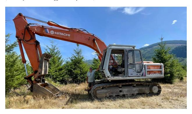
I can't just wait for a disaster to happen and then expect these machines to work. I have to prepare. Last week I did equipment maintenance including charging all the batteries, topping off all the fluids and fuel, and making sure they all start and run. I do all this every quarter but made a special effort last week as I knew this set of storms was coming.
